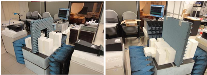
Figure 7 – Setup for the experimental macroscopic characterization of Eccosorb AN-75
